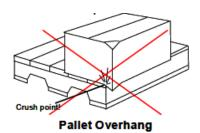
Pallet overhang can reduce compression strength by up to 32 percent.
